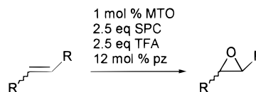
Figure 1. Mode of activation of MTO by SPC/TFA for epoxidation of olefins.
